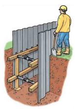
Trench sheets with timber walings, screw props, puncheons and sole plates
