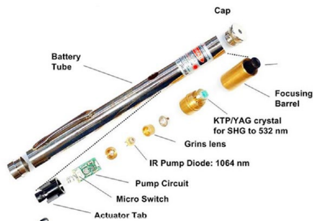
Figure 3. Schematic of a green laser diode pointer.
