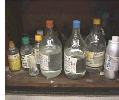
These chemicals are not segregated properly – there are strong acids being stored next to strong bases, and oxidizing acids (nitric acid) being stored with flammable liquids.
